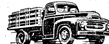
Three light-duty stake models. 7 1/2 and 8 1/2-foot bodies. GVW ratings 4,200 to 8,600 lbs.
