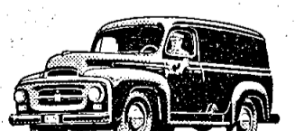
Six panel models. Inside body length 90 inches. All-steel body. GVW ratings 4,200 to 6,500 lbs.
